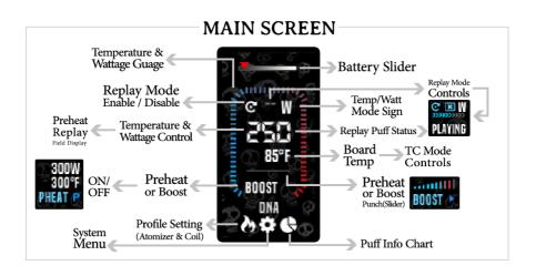
The **power** field is displayed in a large font that supports **power**, **temp and replay modes**. There is an icon in front of the coil material in Portrait & SG (replay text as a button on other versions) to **activate** the **replay** mode. By activating the replay mode, the **power field gets smaller**, the **slider** and other replay mode requirements are **displayed** (Replay Warmth, Lock and Playing).
