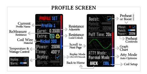
The profile setting screen information is displayed in **two pages**, by pressing the button key at the bottom of the page you will be redirect in next page screen. Here is also a separate page to display the information
