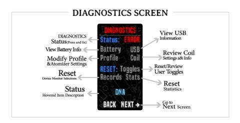
By pressing the **"Next" Button** on the **bottom of the screen** you can **find more** information for **Diagnostics** include Always On Status, Connection Status, USB Charge Current, USB Charge Power, Total Puffs Time and Count, Reset Counts and Device Research Seal Status.
