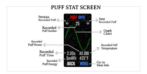
By pressing the "**More**" Button on the bottom of the screen you can find **fully information of recorded puffs without connecting to pc** include: Recorded Puff Time and Date, Recorded Puff Duration Time, Recorded Puff Energy, Recorded Puff Power, Recorded Puff Temperature and Recorded Puff Peak Temperature.
