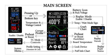
In the **DS** and **Gold** versions, the **graphic design** is **bolder** with displaying enough information and in the **SG version** tries to maintain the simple appearance of the portrait version, with the difference that a large slider is displayed around the screen fields and **changes color** with **increasing or decreasing power** or **temperature**.
