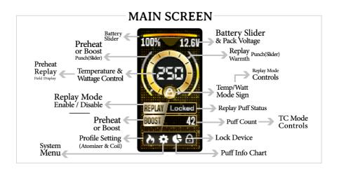
By pressing the "Pheat" text, you will be enable / disable Preheat. You can switch between showing Temp or Punch using the slider, and Power.
