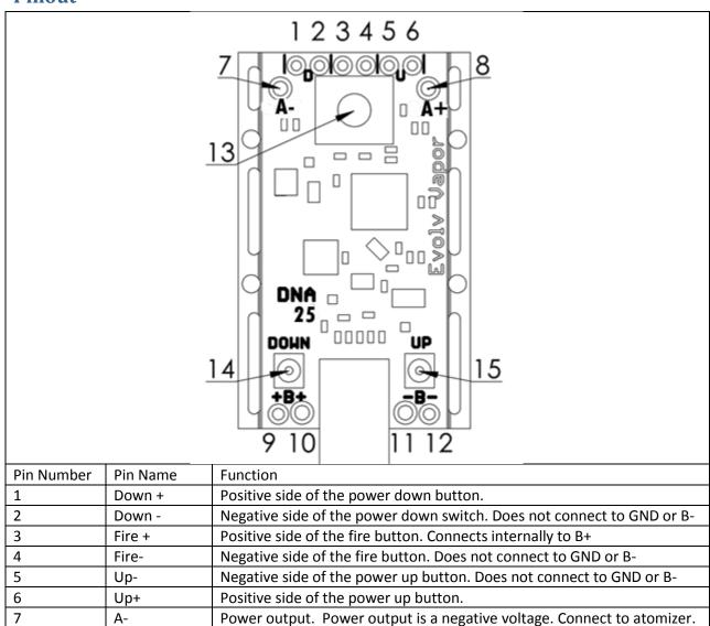
Power output. A+ is the **ground** return for the atomizer. It is connected
