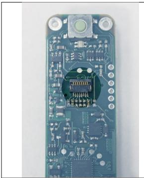
**Step 1:** Locate the ZIF connector on the DNA 75 PCB
